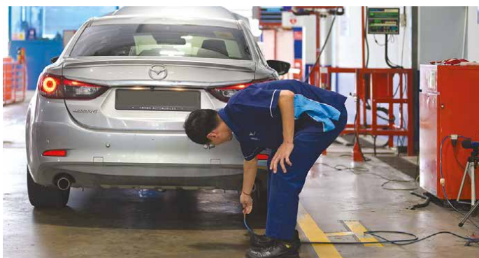
An inspector carrying out emission testing to ensure compliance to regulatory requirements.
