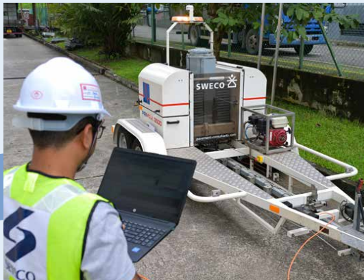
In testing of pavement, SETSCO deploys the heavyweight deflector to determine its loading capability.
