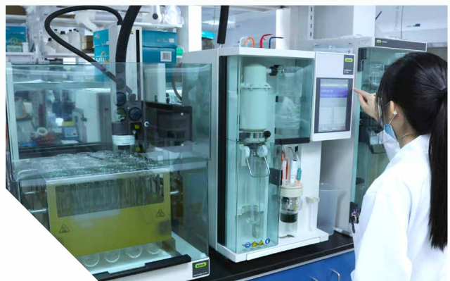
Measuring the amount of protein content in food products.
