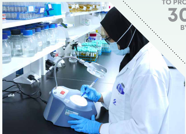
Counting the bacterial colonies to determine food safety.
