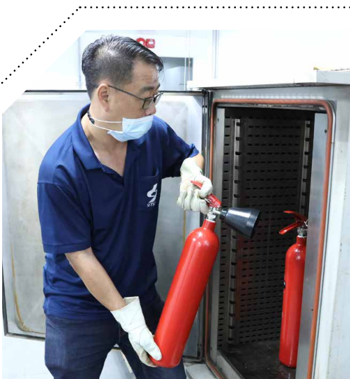
Evaluation of the extinguisher's functionality under extreme temperatures.
